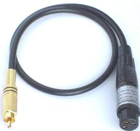
This cable is used to adapt the level, impedance and balance of digital XLR outputs, allowing the PAS-8 outputs to be connected to unbalanced coaxial inputs. Levels, balancing and impedance are converted to standard SPDIF values without any format conversion taking place. Please note that the receiving device needs to be able to process the transmitted format. The cable is usable for sample rates up to 192 kHz. Available lengths: 0.5 m, 1.0 m, 2.0 m and 3.5 m.
