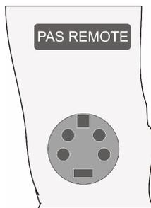
In the pack panel of the digital audio router there is a 4-pole mini DIN socket labelled **PAS REMOTE**. It is used for connecting a serial remote controller. The remote controller has feedback LEDs for all functions.
